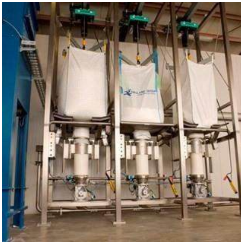
Big Bag losinstallatie
